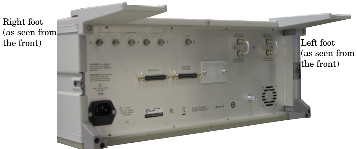
Figure 12 Install Locking Feet on N5261/62A
