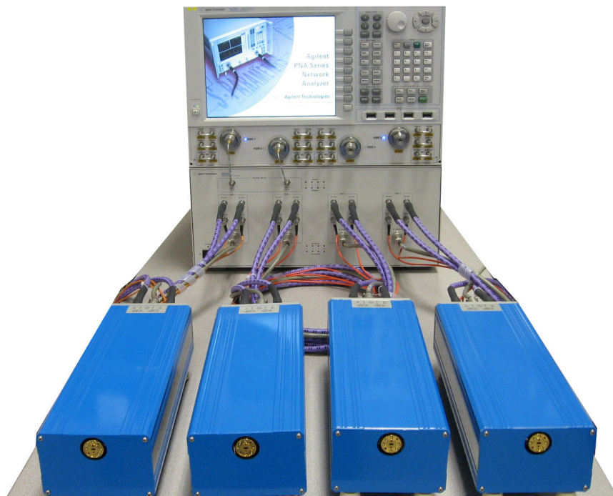
Figure 3 4-Port Banded Millimeter-wave Configuration (N5262A)
